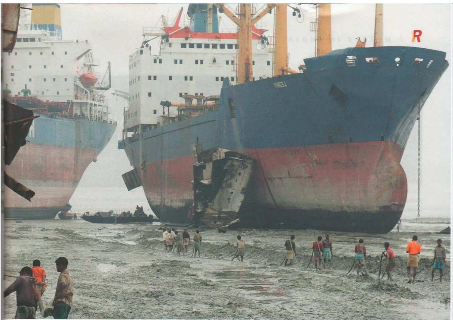
By far the most important source of scrap for India's steel industry is the shipbreaking industry, which accounts for some 11 million tonnes.
